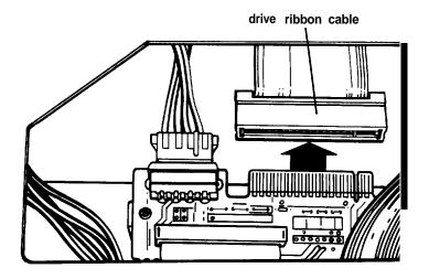
2. Remove the power supply cable from the back of the drive. It is located near the ribbon cable interface, as shown in the next illustration.
